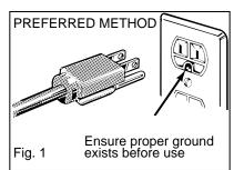
providing an escape wire for the electric current. This appliance is equipped with a power cord having a grounding wire with a grounding plug. The plug must be plugged into an outlet that is properly installed and grounded. (Fig. 1)
